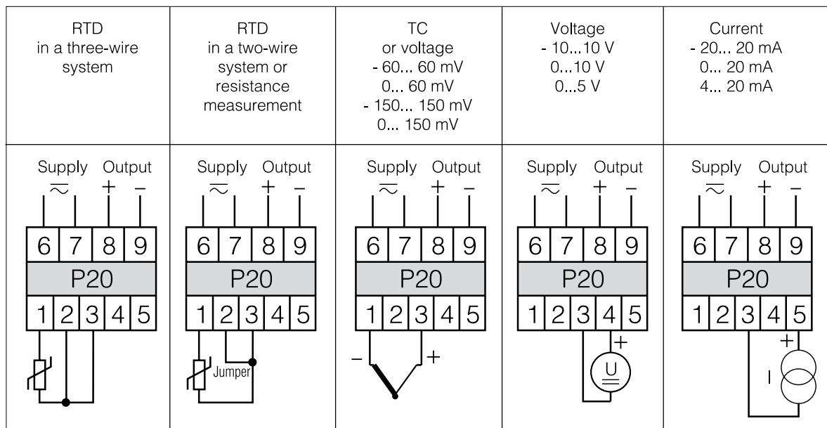
Coding of the P20 transducer input kind
