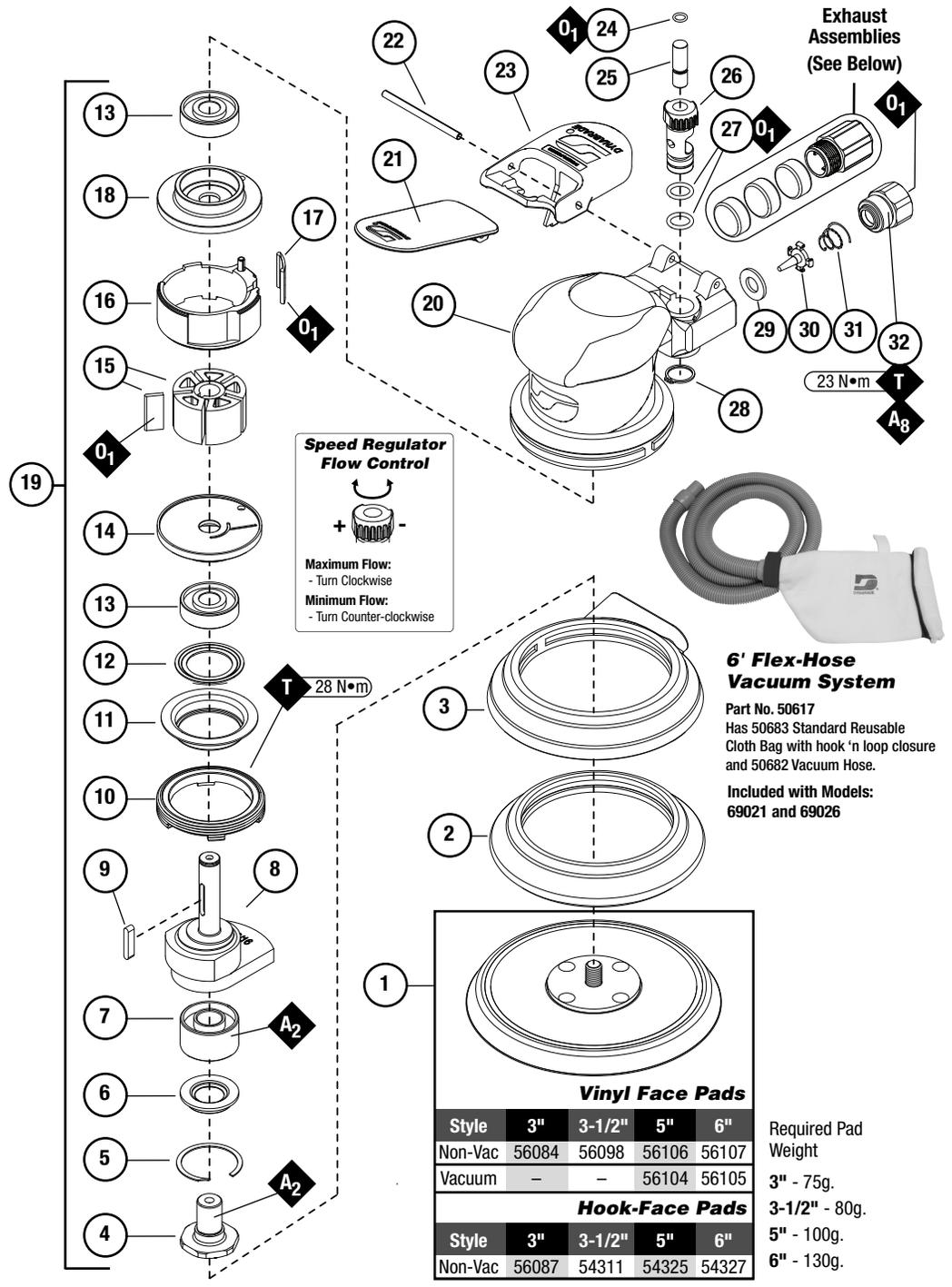
**Note: 56027 Muffler Insert(s) are installed with (1) in the housing body and (2) in the muffler cap . Replace accordingly.**
