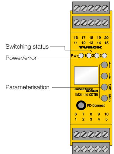
The rotation speed monitor IM21-14-CDTRI analyses frequencies, rotation speeds and pulse trains of rotating motor, gear or turbine parts according to over or undershoot of adjusted limit values. The current value is indicated on a display on the front of the device.
