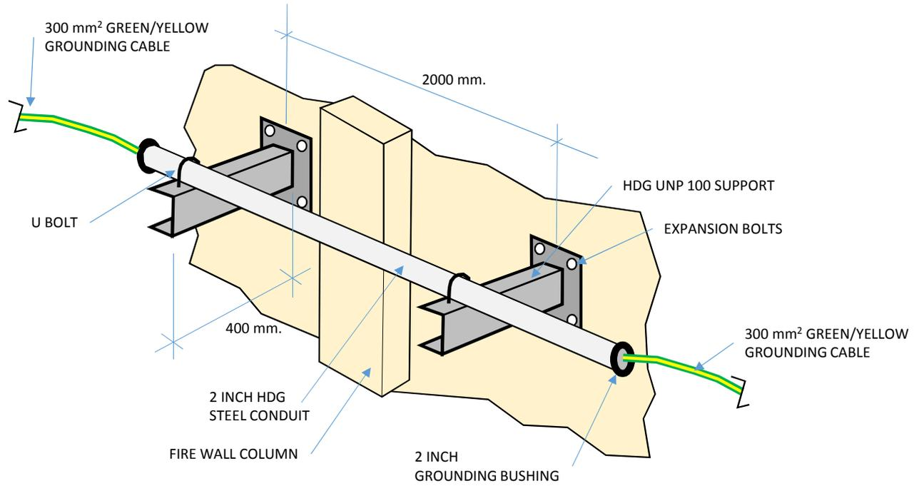
**CONDUIT FIXING DETAIL**
